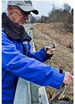
stopwatch at the precise moment the first stick passes exactly under the upstream side of the bridge, then stop the watch precisely when the stick appears at the downstream side.
