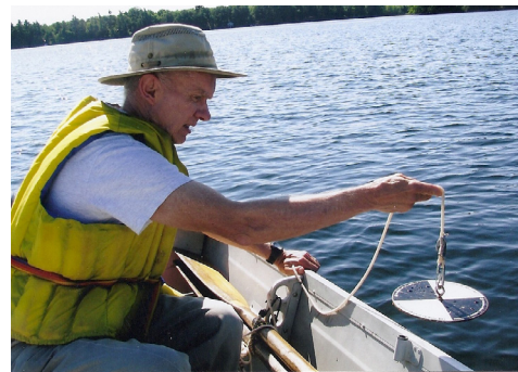
Murray using a secchi disc to assess lake water clarity.
